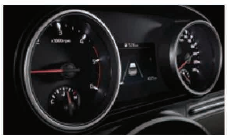
Supervision Cluster (4.2-inch Color TFT LCD)
